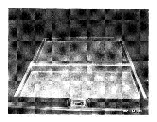
3 Pull off coupler (66) for fuel readout and unscrew immersion tube transmitter (65).
